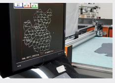
**Cutting and Collecting of cut pieces**: at the end of the cutting phase, the leather is automatically moved to the collecting area. Through a proper pedal the operator can move the cut pieces near his workspace to easily collect them. A projection system highlights the cut pieces with colors and codes, ensuring quick collecting and no errors.
