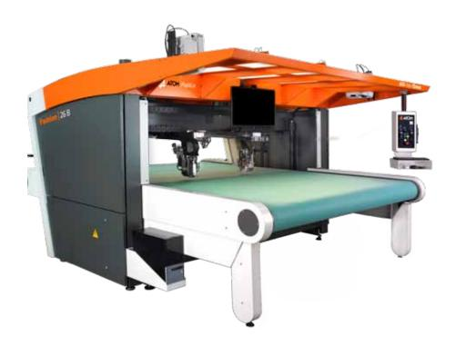
FlashCut Fashion All-in-One models combine processes of acquisition, automatic nesting and cutting in a single machine. Operating in continuous workflow, they both reduce cycle time and allow a single operator to execute all the production steps. Two independent cutting heads ensure the highest productivity in processing both half-hides and full-hides. Made for footwear, leather goods, furniture and automotive upholstery industries.
